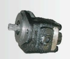
The P21 direct mount gear pump is bi-rotational with side and rear ports for versatility, thus eliminating the drive line for added safety and dependability. This pump has an S.A.E. "B" 2-bolt flange and is used for lighter duty hoists. 10 GPM @ 1200 RPM
